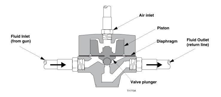
Fig. 1. Cutaway of Pneumatic Back Pressure Regulator
